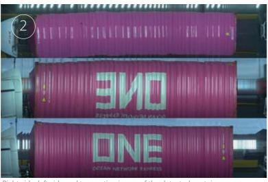
Right side, left side and top section image of the detected containers
