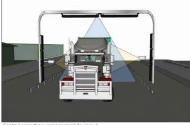
Container section camera module layout
